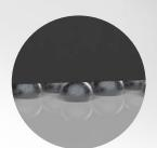
BGA attach to board for greater density and optimized trace breakout region
